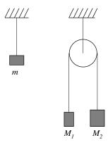
(The first contains a hanging mass m. The second contains a hanging pulley, over which two masses,  $M_1$  and  $M_2$ , hang.) Both supports have acceleration  $a_s$  downward. What should m be, in terms of  $M_1$  and  $M_2$ , so that the tension in the top string is the same in both cases?
