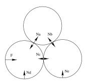
• The low limit on the acceleration is given by the condidtion that the two bottom cylinders lose contact, i.e.,  $N_c = 0$ . Then, the horizontal component of the force on the right cylinder is
