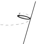
Assume conditions have been set up so that (1) the point of contact between the ring and the cone moves in a circle at a height h above the tip, and (2) the plane of the ring is at all times perpendicular to the line joining the point of contact and the tip of the cone.
