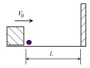
The block's speed is  $V_0$ . The block strikes a particle with very small mass m (and negligible size), which is initially at rest at a distance L from the wall. The particle bounces elastically off the block and slides to the wall, where it bounces elastically and then slides back toward the block. The particle continues to bounce elastically back and forth between the block and the wall.
