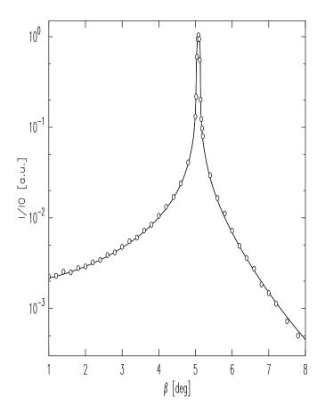
FIG. 3: Diffuse scattering off the liquid Sn surface measured at a fixed grazing angle of incidence  $\alpha = 5.05^{\circ}$  (open circles). The peak corresponds to the specular condition at  $q_z = 0.48$  Å<sup>-1</sup>. The line is the capillary wave theory predictions for surface tension  $\gamma = 560$  mN/m.
