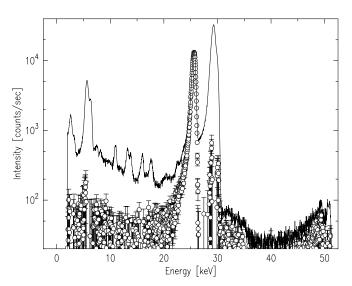
FIG. 7: Raw (line) and background-subtracted (open circles) measured fluorescence from the surface of liquid Sn. The sharp lines are due to the K emissions lines<sup>20</sup> of Fe (E=6.4 keV), Nb (E=16.6 keV), Mo (E=17.5 keV) and Sn (E=25.2 keV).
