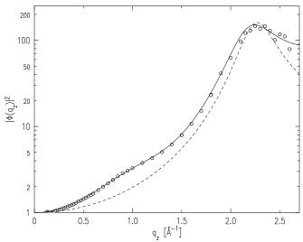
FIG. 4: The structure factor (squared) of the Sn surface as derived from the measured reflectivity  $|\Phi(q_z)|^2 = R(q_z)/[R_F(q_z)CW(q_z)]$  (open circles). The dashed line is the theoretically expected  $|\Phi(q_z)|^2$  of a simple layered density profile as found previously for Ga and In. The solid line is a fit to a model, discussed in the text, where the distance between the first and second layers is reduced by 10% relative to that of the subsequent layers.
