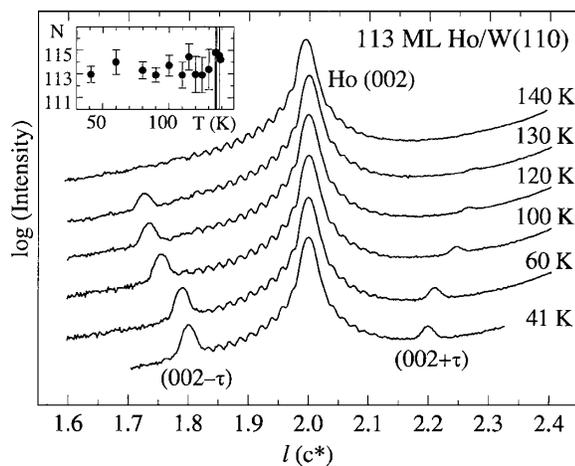
FIG. 1. Resonant x-ray scattering from a 113 ML thick Ho film along the specular (00 $l$ ) direction, recorded in the  $\pi$  channel. The length  $l$  of the scattering vector refers to the reciprocal lattice parameter  $c^* = 2\pi/c$  of hcp Ho. The inset displays the number  $N$  of coherent magnetic planes.
