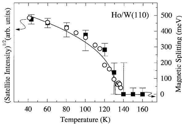
FIG. 4. Temperature dependences of the Ho  $\Delta_2$  splitting (solid squares) and of the square root of the integrated  $(002 - \tau)$  intensity (open circles). The solid line represents a power law with  $T_N = 131.4$  K and  $\beta = 0.39$  (from [5]).
